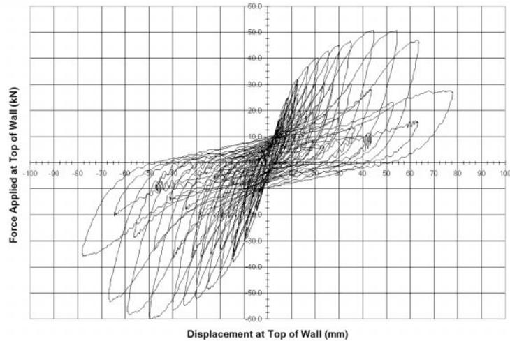
Figure 5: Sample Type C (Pneumatically Driven Common Nails) w/ Reduced Cyclic Displacement, Sequence 3
