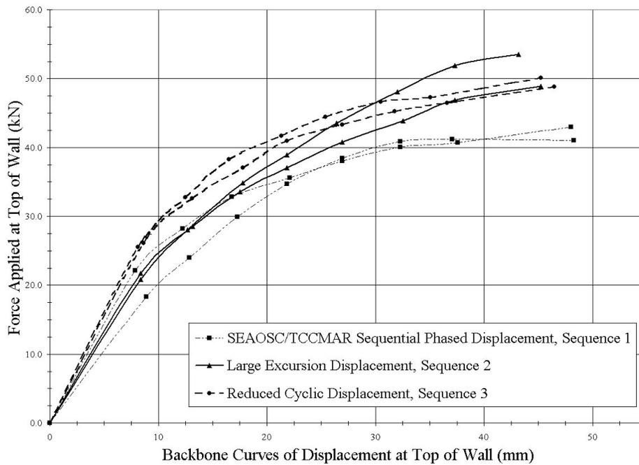
Figure 7: Backbone Curve of Sample Type B (Hand Driven 8d Galvanized Box Nails)
