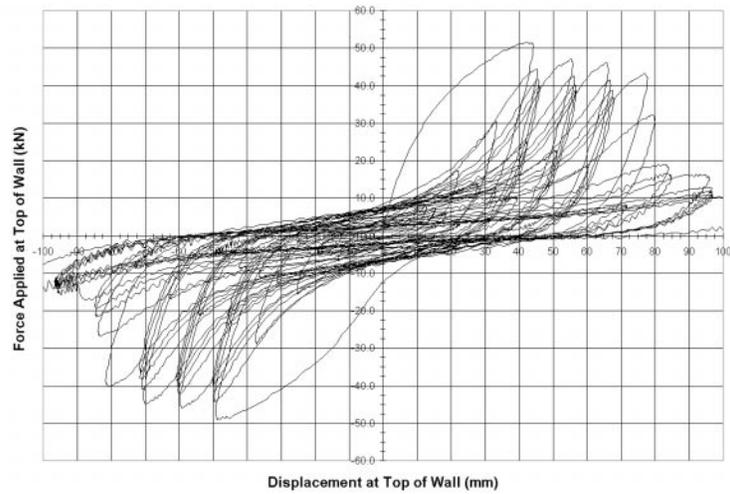
Figure 4: Sample Type C (Pneumatically Driven Common Nails) w/ Large Excursion Displacement, Sequence 2
