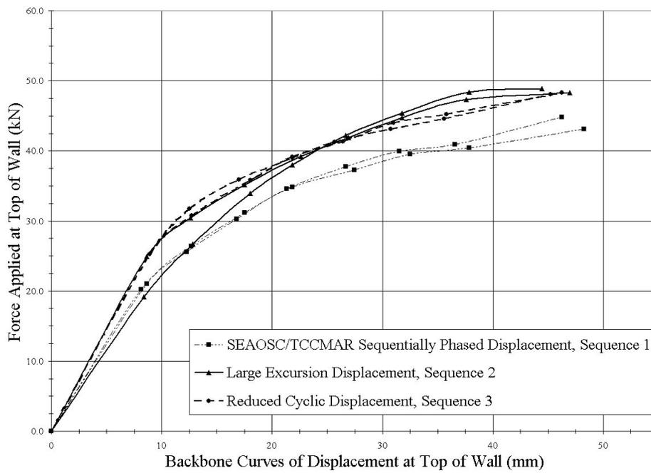
Figure 9: Backbone Curve of Sample Type D (Pneumatically Driven 8d Box Nails)
