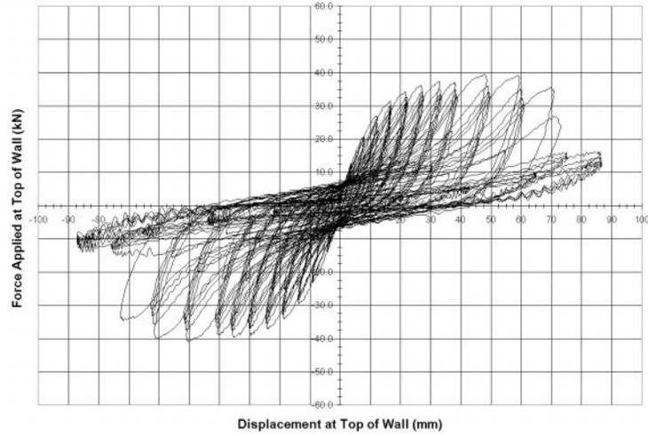
Figure 3: Sample Type C (Pneumatically Driven Common Nails) w/ Sequentially Phased Displacement, Sequence 1
