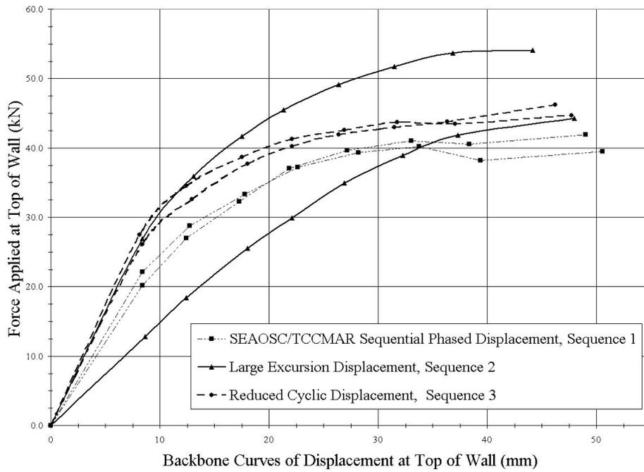
Figure 6: Backbone Curve of Sample Type A (Hand Driven 8d Common Nails)
