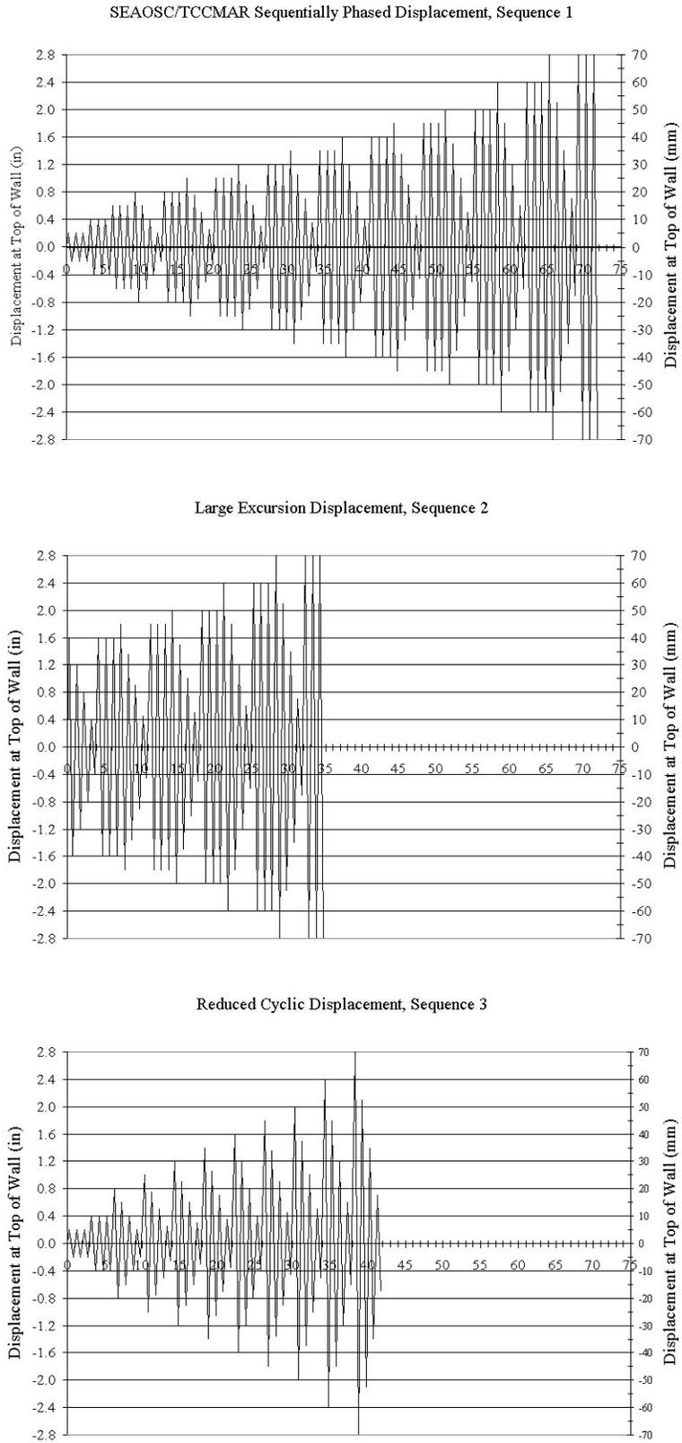
Figure 2. Three Different Loading Sequence Protocols
