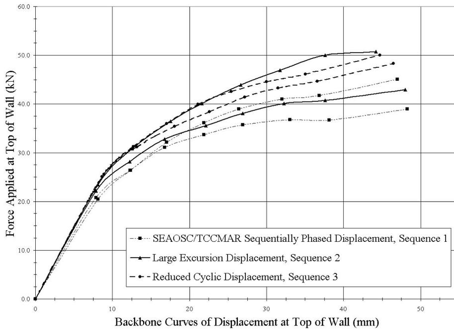
Figure 8: Backbone Curve of Sample Type C (Pneumatically Driven 8d Common Nails)
