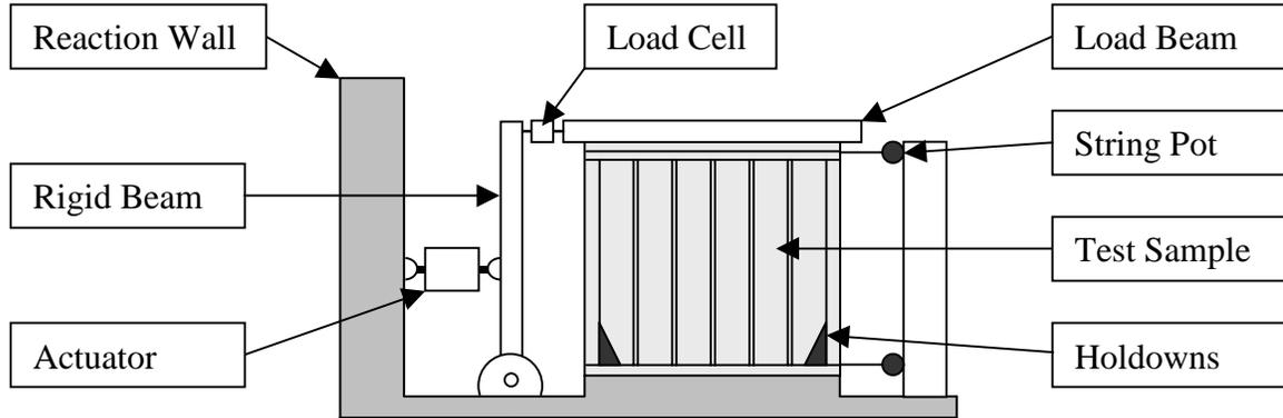
Figure 1: Test Set-up
