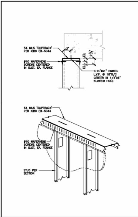
**Figure 3:** Slotted Slip Track Joint Detail
