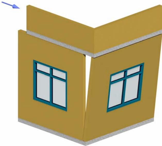
**Figure 9:** Corner Incompatibility at Floor-to-Floor System
