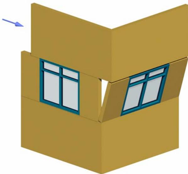
**Figure 10:** Corner Incompatibility at Spandrel System
