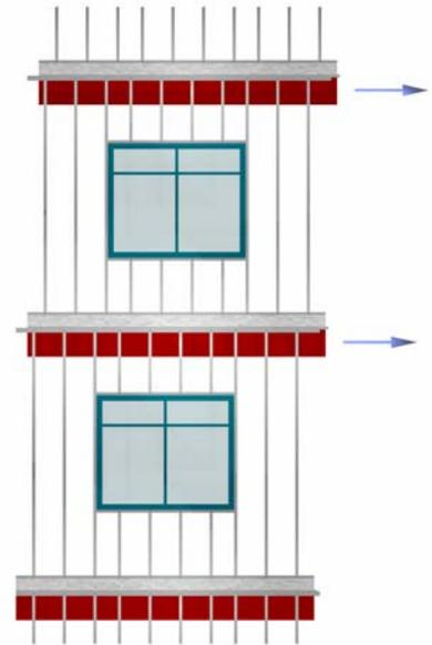
**Figure 5:** In-Plane Movement of Floor-to-Floor Framing System
