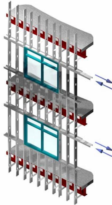
**Figure 2:** Typical Spandrel System with Joint at Head of Window
