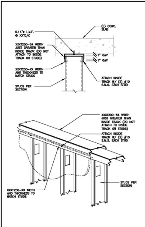
**Figure 4:** Track Within a Track Joint Detail
