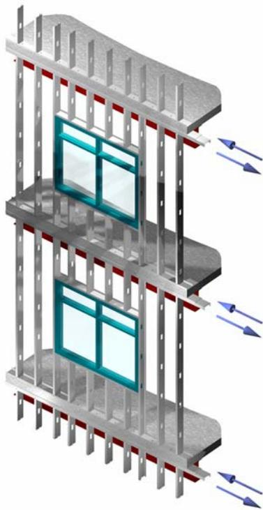
**Figure 1:** Typical Floor-to-Floor Framing with Joint Below Floor Line
