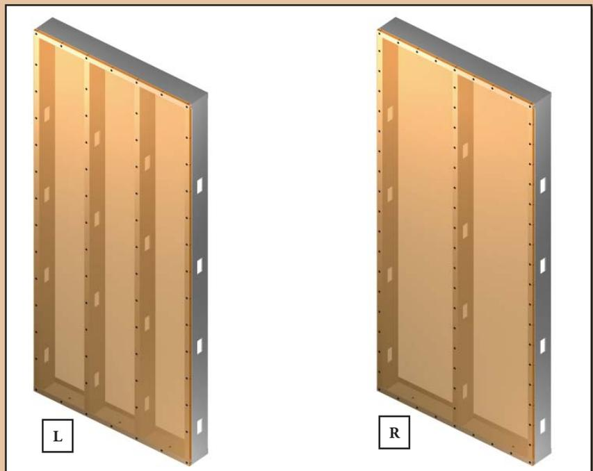
Typical 4 foot wide sheathing with 16-inch on center studs (left) and 24-inch on center studs (right)
